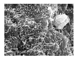
SEM image of carbanionic CNTs coated with PMMA
