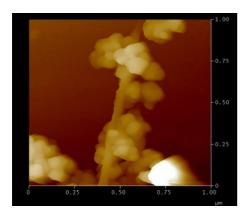
AFM image of MWNT partially coated with nanozirconia
