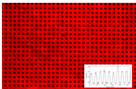
Figure 1) Fluorescence microscopy image of a Streptavidin–Texas Red pattern on Glass obtained by microcontact printing technique (motives size is 5µm).
