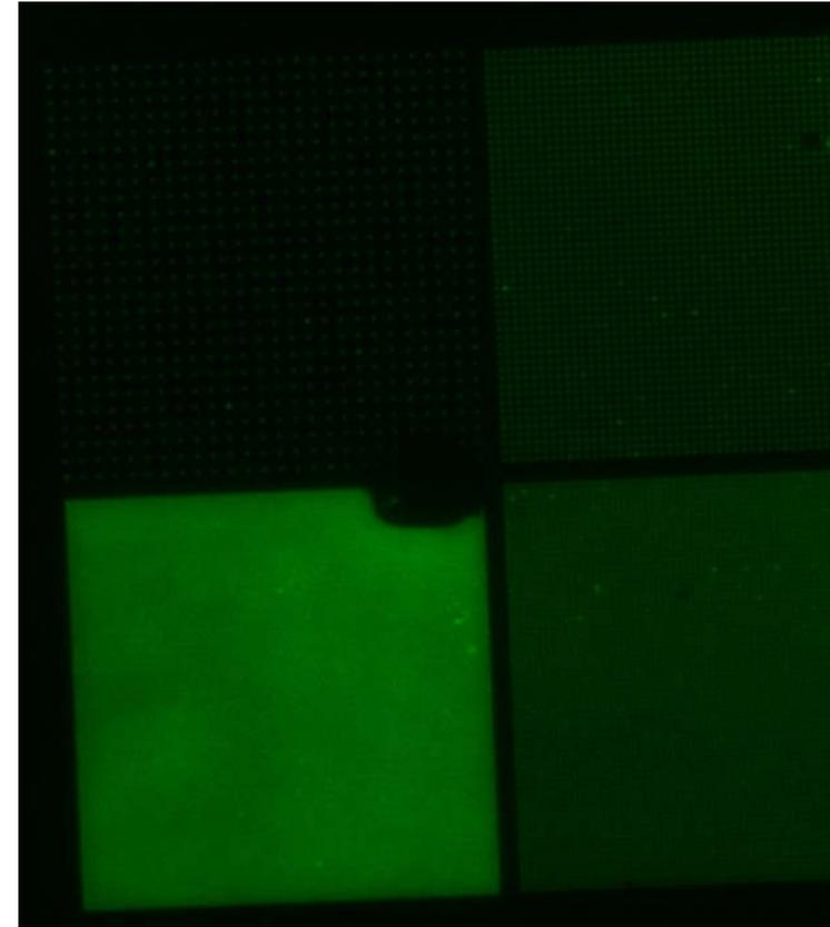
Nanopillars ( $h = 100\text{nm}$ ,  $d = 100\text{ nm}$ ) of stabilized PAA on PEO-like
