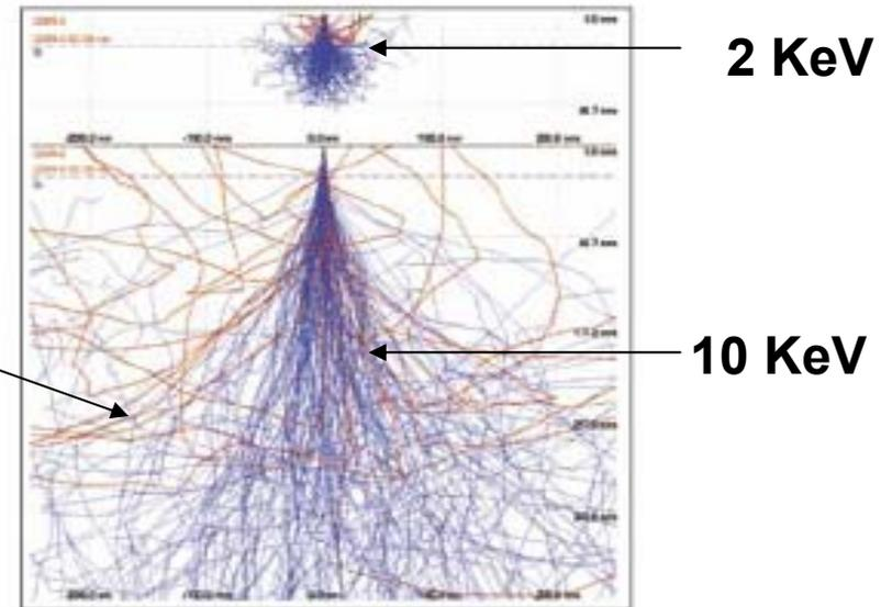
Figure 1: Simulation of electron scatter for 2 keV and 10 keV
