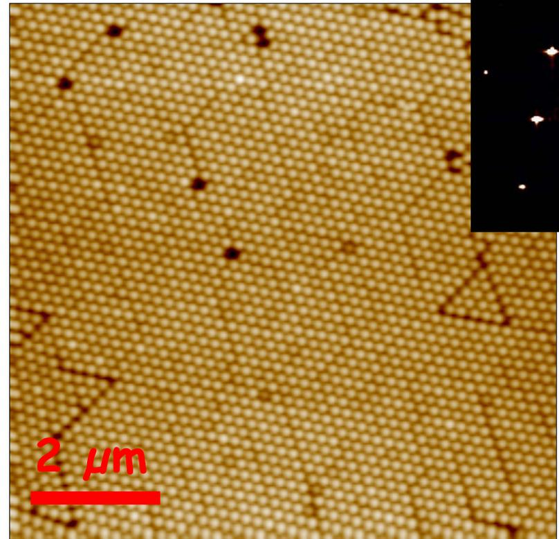
Fast and cheap. Nano-sphere Surface coverage up to 95 % over  $\text{mm}^2$ . Polycrystalline hexagonal monolayer of nanospheres
