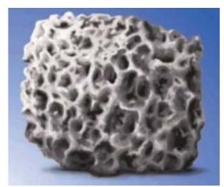
*Figure 4.* PLLA scaffold obtained by thermally induced phase separation
