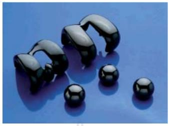
**Figure 1**. Diamond Like Carbon biocompatible coatings on hipjoint and knee artificial implants
