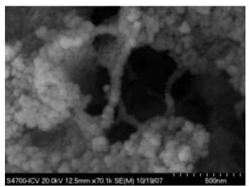
Figure 5 MWCNT coated with nanozirconia obtained by hydrothermal synthesis
