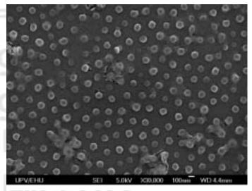
Figure 8. Dispersion of NIPAM nanogels on a Si substrate
