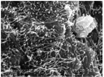
Figure 6. PMMA wrapping SWCNTs
