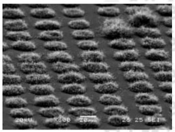
Figure 7. MWCNTs grown on a patterned Si substrate
