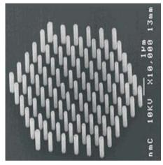
Fig 11. Epitaxial InAs nanowires grown on a Si(111) substrate from holes etched in a SiO2 film.
