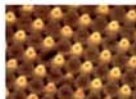
AFM image of a two dimensional crystal of the bacteriophage F29 connector
