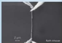
Direct 4-contact nanoprobing of an Au-capped Ni/NiO nanowire
