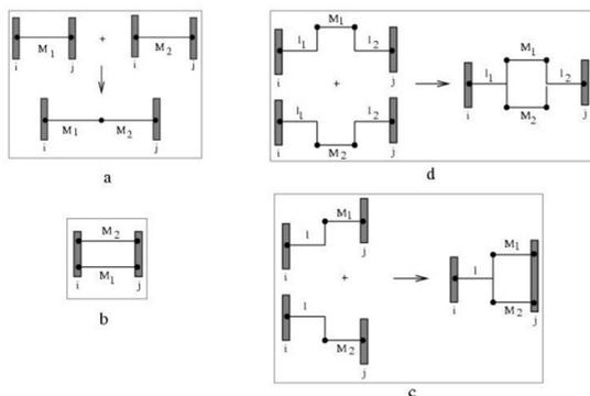
**Fig. 1** > Simple single molecule circuit diagrams represented with their two contact nanopads metallic interconnects of the different series and parallel association of the molecular wires  $M_1$  and  $M_2$ . The two molecular wires are: (a) bonded in series, (b) connected in parallel on the metallic pads, (c) forming a single molecule with one intramolecular node and (d) forming a single molecule with two intramolecular nodes./
