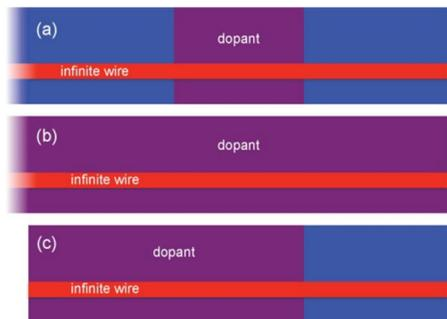
**Fig. 5** > Scheme for the atomic structures that held a wire over three different Si surface region: two semi-infinite electrodes and a central connecting region between the electrodes. In (a) only the central region is doped, in (b) there are dopants in the three regions, and in (c), dopants are found in two regions, one being the contact region./
