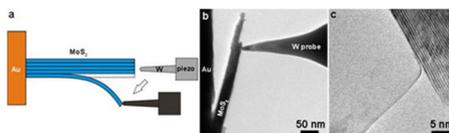
**Fig. 1** > Nanomechanical cleavage of molybdenum disulphide atomic layers. (left) Schematics of the experimental setup inside HRTEM. (center) TEM image of a sharply etched tungsten nanoprobe in contact with the  $\text{MoS}_2$  single crystal deliberately placed with (0002) basal atomic planes viewed edge-on. (right) HRTEM image of a cleaved  $\text{MoS}_2$  atomic monolayer./
