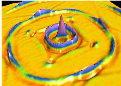
**Fig. 4 >** Experimental image of surface acoustic waves on a crystal of tellurium oxide./
