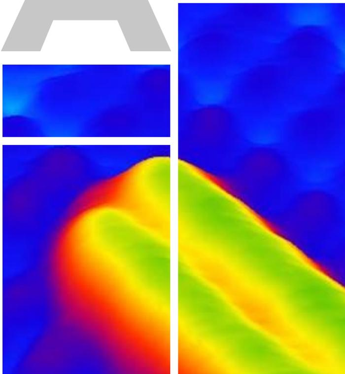
*Atom by atom constructed dimer dangling bond wire on an Si(100)H surface*
