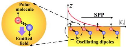
**Fig. 2 >** Generation surface phonon polaritons (SPP) by the fluctuation of electrical dipoles, which under a thermal excitation emit an electrical field that propagates along the material interface. These dipoles are spontaneously present in polar materials as  $\text{SiO}_2$  and  $\text{SiC}$ .
