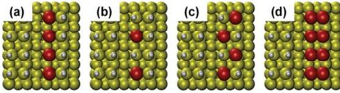
**Fig. 4 >** Atomic structures of (a) the single-row, (b) the half-row, (c) the zig-zag, and (d) the double-row dangling-bond (dangling-bond) wires. H atoms are depicted in white, Si atoms in yellow and red when holding a dangling-bond./
