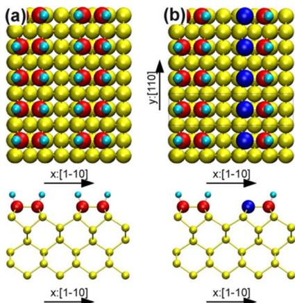
**Fig. 1** > Atomic structure of (a) the Si(100)-(2x1)-H surface, (b) the infinite ideal wire drawn along the y direction. H atoms are depicted in cyan, while Si atoms are depicted in red (surface dimers), yellow (others) and blue when holding a dangling-bond./
