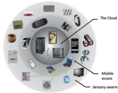
Fig. 1 > The hierarchy of emerging network of communicating systems consists of a layer of various sensors monitoring environment, health, safety etc. connected to mobile phones, tablets and other mobile applications and to the cloud. All the layers benefit from thermal management leading to low power consumption and from energy scavenging facilitating the expansion of the swarm [1]./
