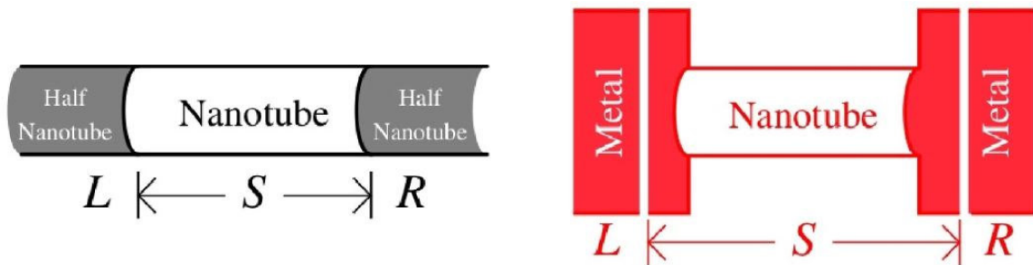
Figure 3.1: Quantum transport : modelisation of the contacts between a carbon nanostructure.
